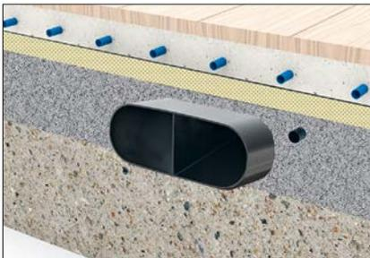
Shallow duct in the balancing layer (acc. to DIN 18560-2)
